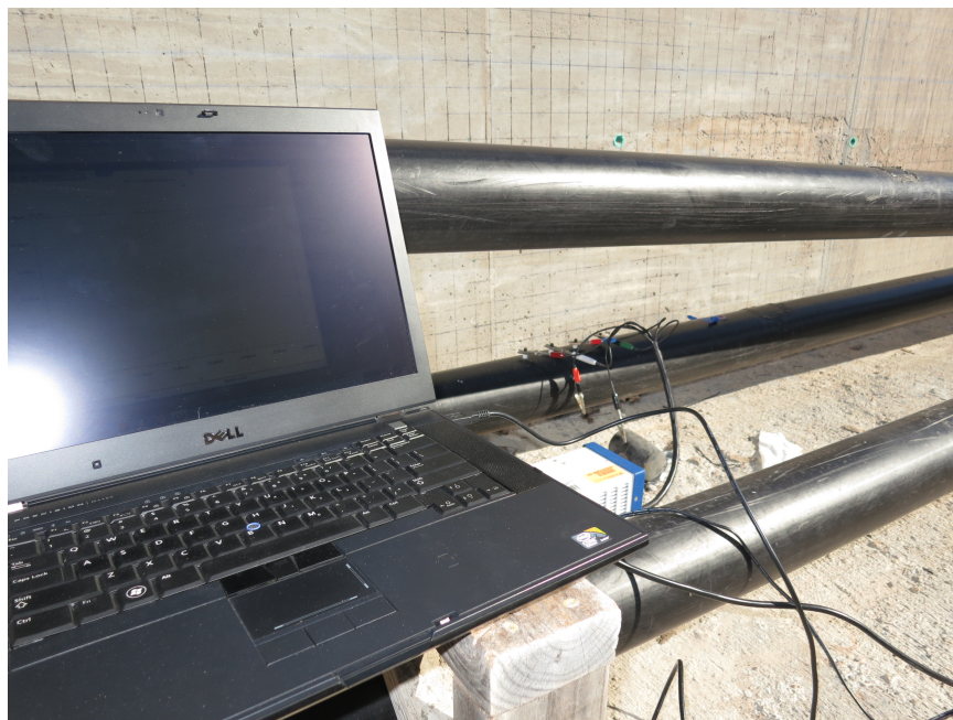
Figure 3.6: Experimental setup of the indirect impedance measurement. Photograph taken at the Texas A&M mock bridge by Mark Orazem. The Gamry Reference 600 potentiostat is the white/blue box in the center of the photograph.
