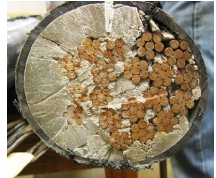
This section of a bridge tendon shows the thick outer wall of the duct and the cables embedded in grout on the inside.
